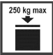
Stacking weight limitation (Shown here is 250 kg)
