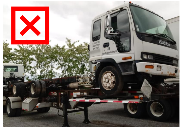
Cargo loaded on container chassis not acceptable
